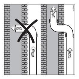
If the exhaust is ducted into an inactive flue, the air must be expelled parallel to the flow direction of the flue. Never connect an exhaust hood to an active chimney, dryer vent, vent flue, or room venting ductwork. Seek professional advice before connecting an exhaust hood vent to an existing, inactive chimney or vent flue.
